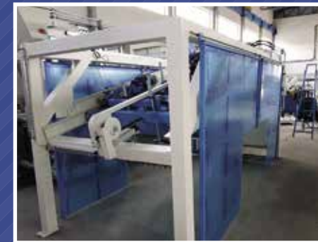
Equipment for decorative processing of surface of concrete products (paving stones, pedestrian blocks, etc.) with water supply under high pressure
