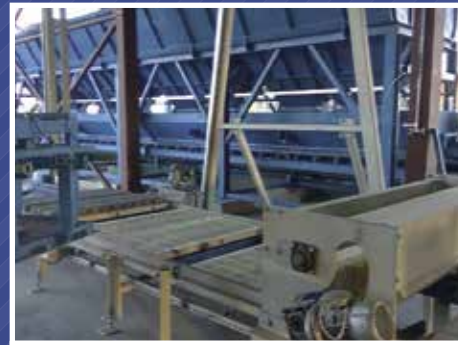
Rotating brush for wooden pallets cleaning
