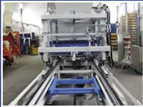
Transport of fresh concrete blocks from the machine with speed/start stop ramp regulation, consists from two chain transport systems
