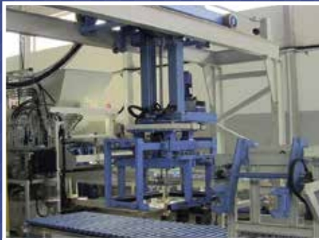
Automatic hydraulic Cuber - the equipment for packing concrete products from production boards to transport boards with hydraulic clamp and electrical lifting -moving of clamp mechanism
