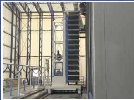
Automatic finger-system – automatic robot-machine to move fresh products after vibropressing from elevator in the drying chamber and back to loverator
