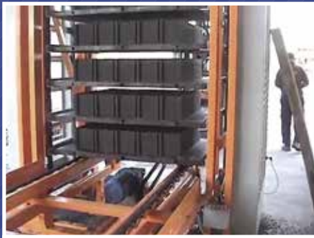
Elevator is an automatic device for accepting and raising pallets with fresh pieces – robot for putting pallets with fresh products into the curing rack (with 6-12 levels for blocks or the 2x 6-12 levels for paving stones)
