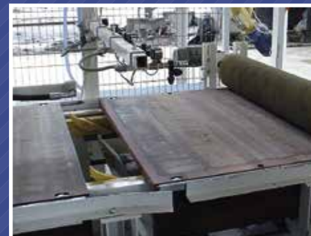
Device for spraying of working pallets
