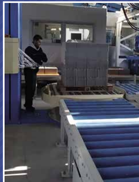
The packing machine for pallets with finished products
