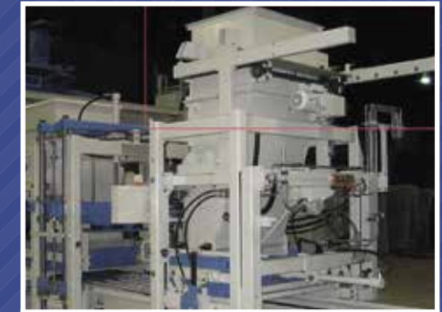
Multicolor or Color mix device allowing to produce a face layer of products with different colors or combinations of mixes
