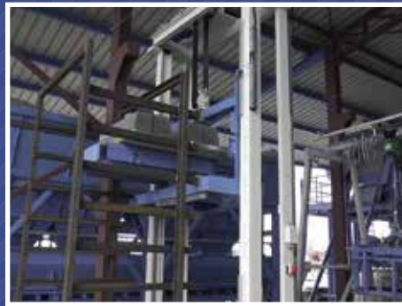
Loverator is an automatic device - robot for accepting pallets with dry products from racks and lowering to transport conveyor to cubing position (with 6-12 levels for blocks or 2x 6-12 levels for paving stones)
