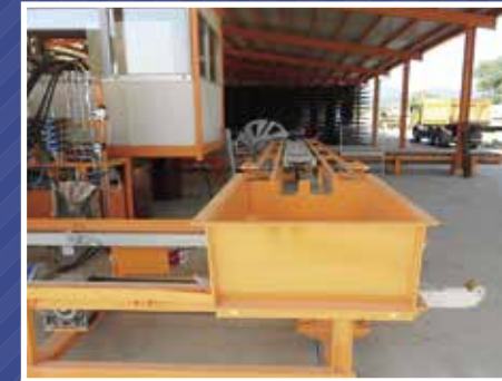
Pallet insert device with pallet magazine with soft start/stop and speed regulation
