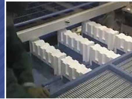
Additional equipment for polystyrene (insulating part of the block)
